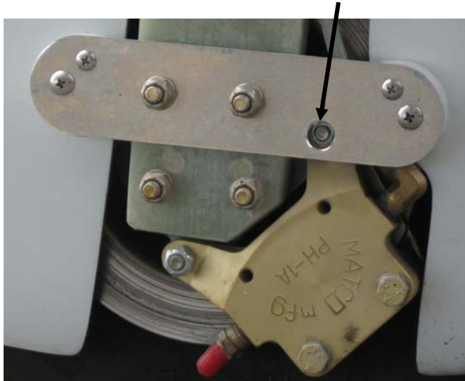
Figure 3: Completed relief hole with wheel and pant reinstalled.
