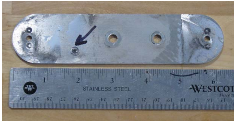
Figure 2: Mark on outside of right-hand inner wheel pant bracket caused by contact with caliper bolt.
