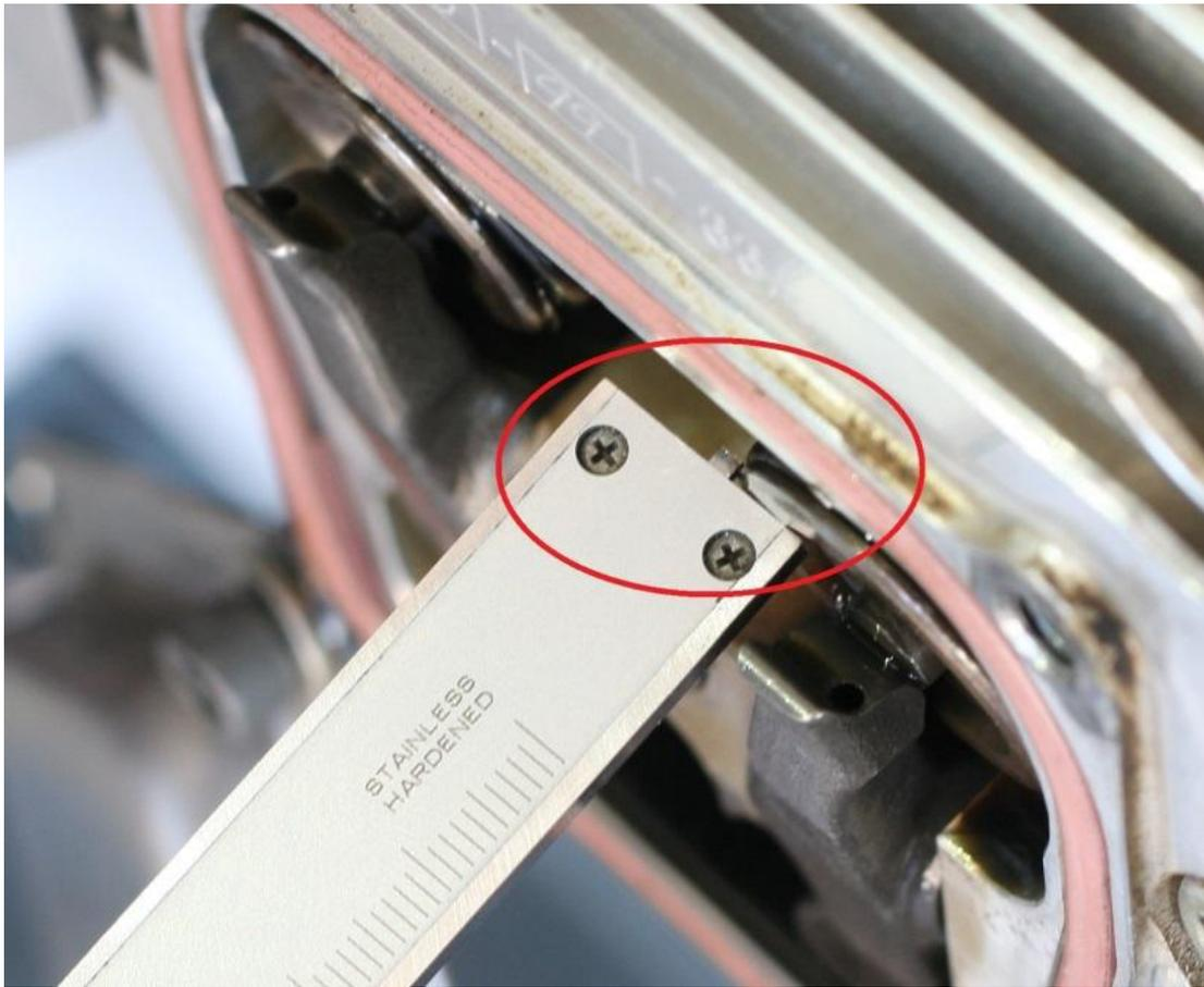
Figure 4 – Vernier Depth Caliper
