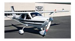
The U.S.—built, Australian-designed Jabiru J230 is a high-wing airplane that's powered by a 120 hp, six-cylinder Jabiru 3300 engine.
